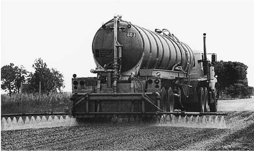
Figure 2.59 Typical liquid calcium chloride spreader for dust control or road stabilization (Dow, 1999, courtesy of The Dow Chemical Company).
