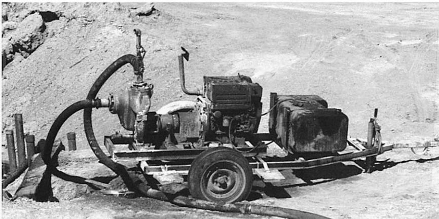
Figure 2.48 Typical brine pumps utilized at Bristol Lake. Top, brackish well at the edge of the lake. Bottom, portable transfer pump for the trenches, pits and ponds. (Courtesy of National Chloride Company of America).
