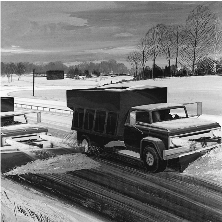
Figure 2.56 Trucks removing loose snow and ice, and spreading salt pre-mixed with calcium chloride (Allied, 1980).
