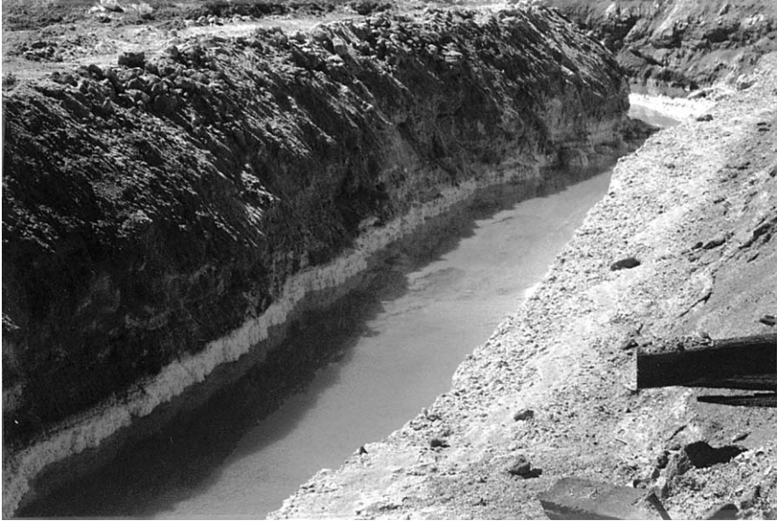
Figure 2.47 A typical brine seepage trench at Bristol Lake (Courtesy of National Chloride Company of America).
